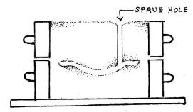
6 MOLTEN IRON IS POURED INTO THE SPRUE HOLE.
